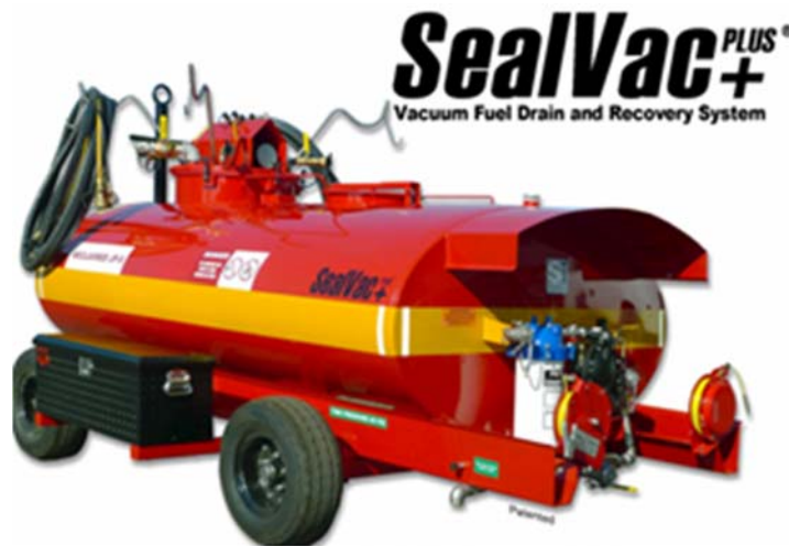
Figure 5-2: SealVacPlus® Vacuum Fuel Drain Bowser and Recovery System
